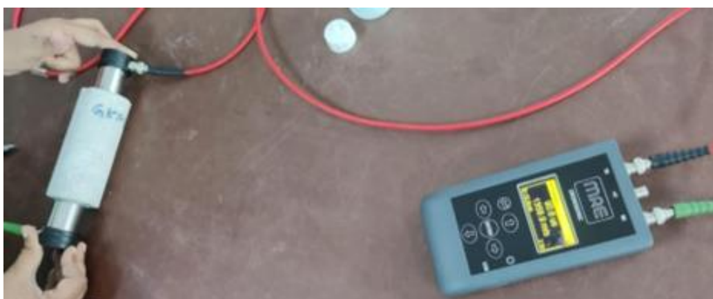
Figure 4: Measurement of P-wave velocity of limestone rock.
