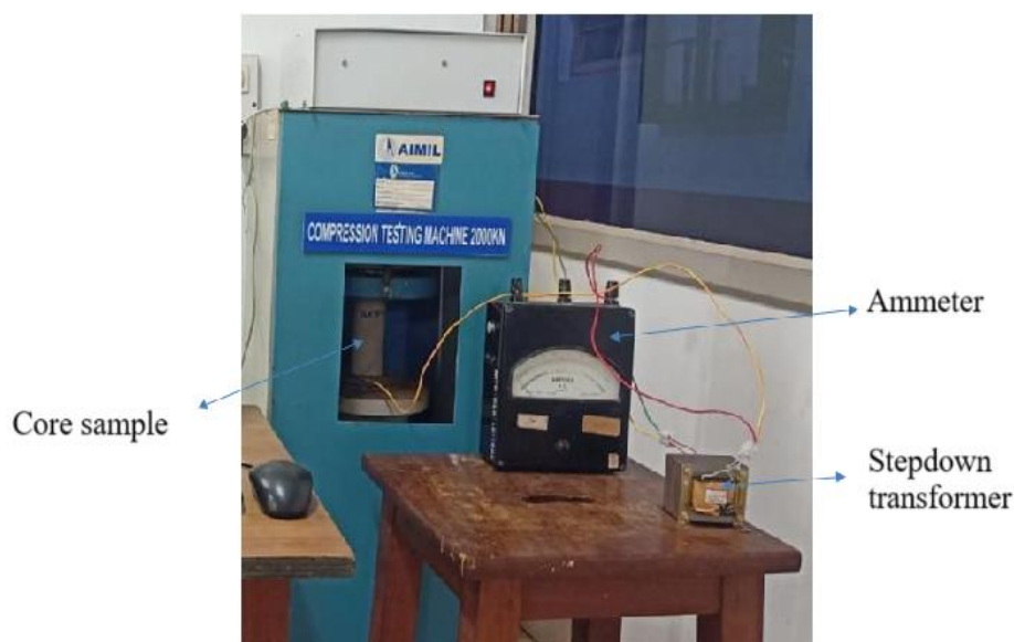
Figure 2: Resistance measurement setup for rocks
